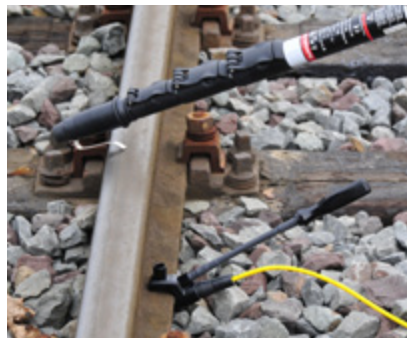
Fast self-test for device function and contact between terminal and rail MultiSafe TT 3K - with rail foot clamp
