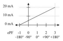
Power angle represents angle between first voltage harmonic and first current harmonic for each individual phase. Total power angle is calculated from total active and reactive power (see equation for Total power angle, chapter *Equations* on page 53). A positive sign shows inductive load, and a negative sign shows capacitive load.
