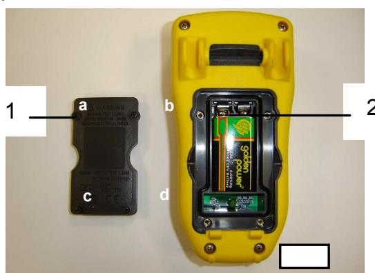
*Figure 6 : access to the battery*
