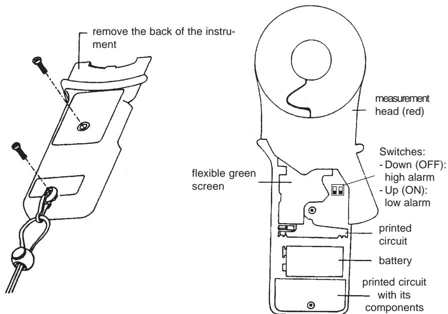
According to the type of alarm selected, crossing of the alarm threshold will be indicated by the appearance of or and a continuous beep at high or low frequency.
