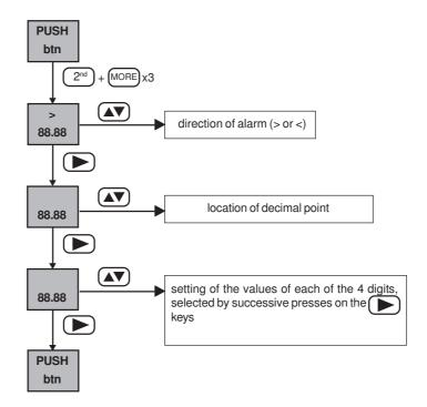
$\Rightarrow$  If necessary, activate alarm threshold I<sub>ALARM</sub> by pressing the **ALARM** key.
