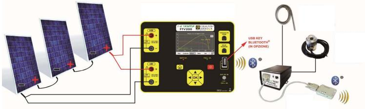
Example of electrical connections with remote unit
