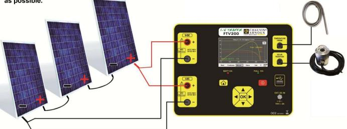
Example of electrical connections without remote unit
