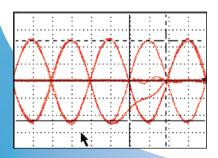
Eye diagram: an advantage for recurrent data display. The traces are cumulated on screen, alternating the trigger-edge polarity.
