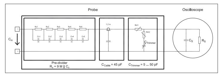
Schematic diagram of a passive 10:1 test probe
