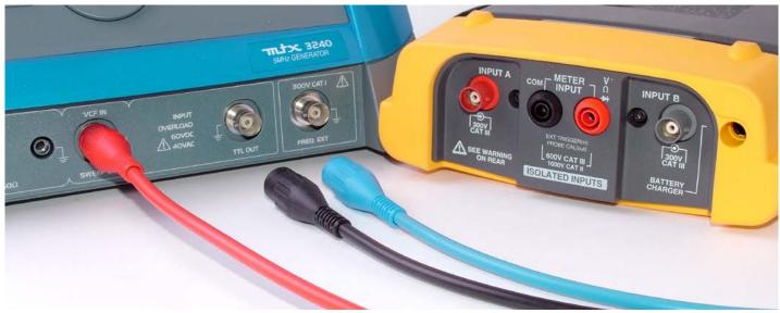
Test leads with touch-protected BNC plugs can be connected to devices with insulated and conventional BNC sockets.
