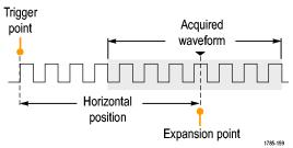
3. With Delay set to On, the trigger point is disconnected from the expansion point. Turn the Horizontal Position knob to move the trigger point away from the expansion point (center graticule). The amount of delay is shown in the Horizontal Status area at the bottom-center of the graticule, referenced to 0 s (center graticule). The trigger point can move off the screen; when this happens, the trigger marker changes to show the direction of the trigger point.
