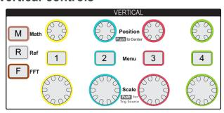
The Vertical controls set the vertical settings (position and scale) for each channel, and enable turning on or off individual waveforms.
