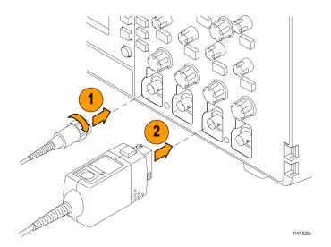
2. Tektronix Versatile Probe Interface (TekVPI®): Push the probe base into the channel connector until the probe base connector clicks. To remove, push and hold the button on the probe base and pull the probe from the connector.
