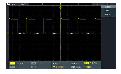
7. Check the shape of the displayed waveform to determine if the probe needs adjusted. If the waveform has a square leading edge and a flat top and bottom, the probe does not need adjusted.
