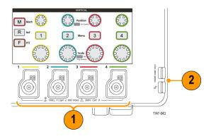
2. PROBE COMP. A square wave signal source and ground connection used to compensate probes.
