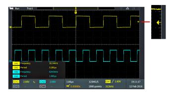
The Time and Date readout shows the oscilloscope clock setting. (See page 10, Changing the date and time.)
