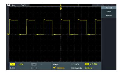
If the displayed square wave tops are not flat, perform the procedures to compensate the probe high frequency response. You can compensate the probe after completing this functional check. (See page 16.)
