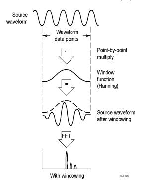
The different window shapes are trade-offs between frequency accuracy and magnitude accuracy. What you want to measure, and your source signal characteristics, help you to select which window to use. Use the following guidelines to select the best window for your signal analysis needs. The Hanning window is a good starting point for FFT measurements.
