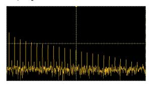
Use the **Linear RMS** vertical scale to see an overall view of how all frequencies levels compare to each other.
