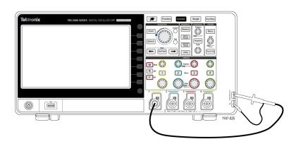
5. Push **Default Setup**. Default Setup returns the oscilloscope settings to factory default values. (See page 111, *The default oscilloscope settings (Default Setup)*.)
