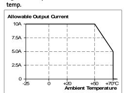
Fig. 15-1 Output current vs. ambient
