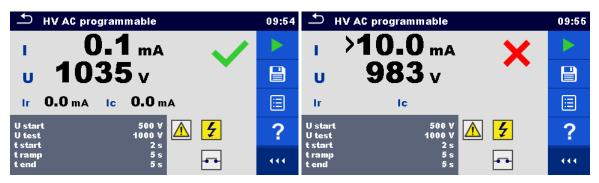
Figure 6.31: Examples of HV AC programmable test results
