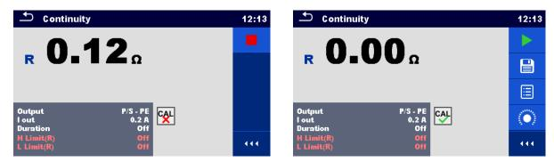
Figure 6.21: Uncompensated and compensated result
