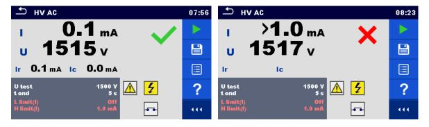
Figure 6.24: Examples of HV AC meaasurement results
