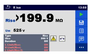
Figure 6.5: Single test result screen
