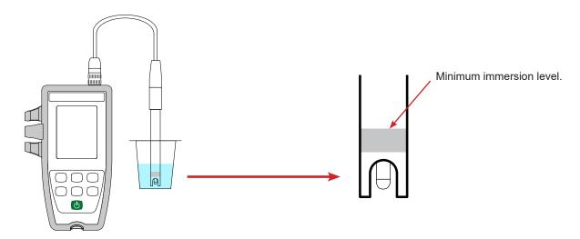
The electrode (optional) has an integrated temperature probe. There is therefore no need to measure the temperature of the solution.
