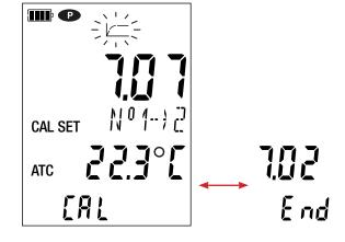
■ If you need only one calibration point, long-press the **END** key. Only the offset of the electrode will be calculated; the slope will be left unchanged.
