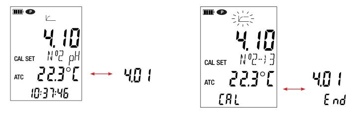
■ If two calibration points are enough, long-press the **END** key. The slope and offset of the electrode will be calculated and displayed. However, you can continue the calibration on a third and last point by pressing the **CAL** key again.
