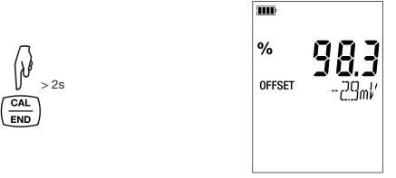
During the calibrations, the slope and offset of a given electrode must not vary more than a little. If you observe a large variation, redo the calibration. If the problem persists, check the buffer solution (in particular the use-by dates) or replace the electrode.
